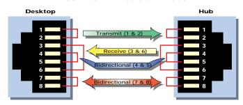
**Note:** Like 10BASE-T, 100BASE-T transmit/receive crossover is in the hub. RJ-45 connectors are shown here.
